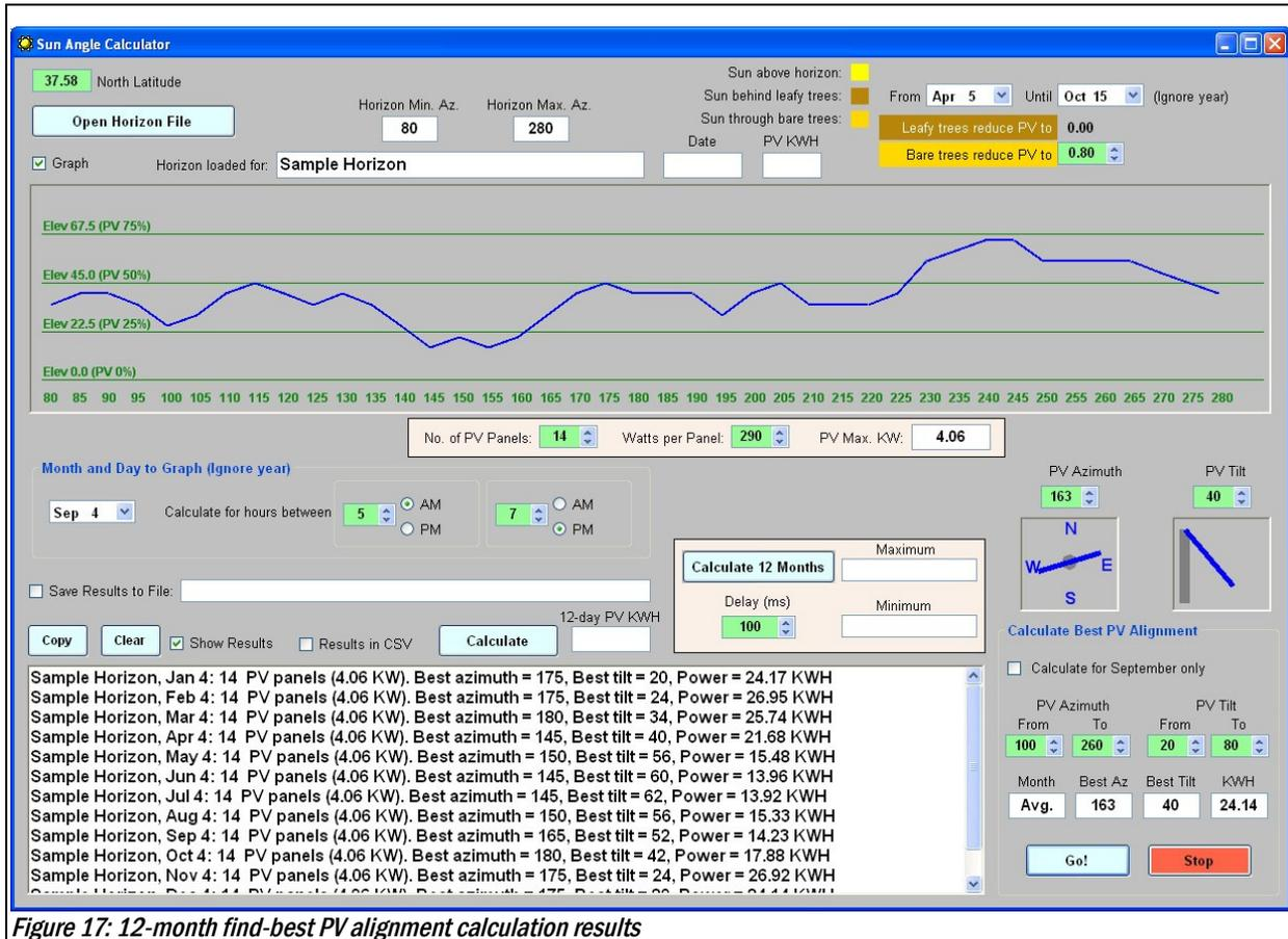
Figure 17: 12-month find-best PV alignment calculation results
