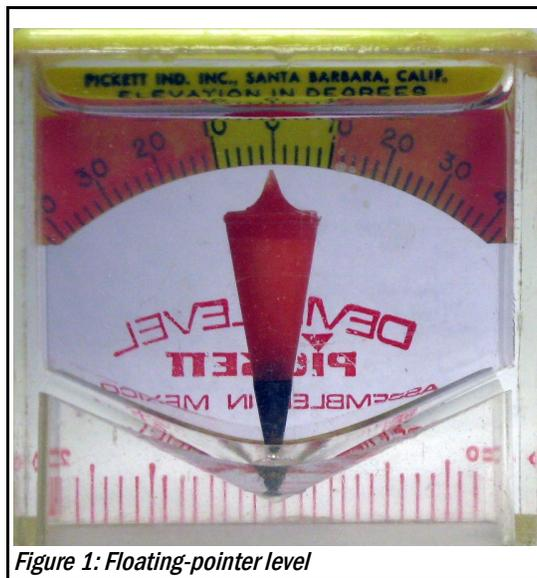
Figure 1: Floating-pointer level
