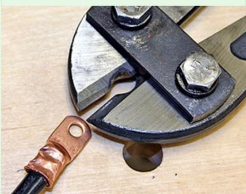
Figure 30: Homemade lug crimping tool
