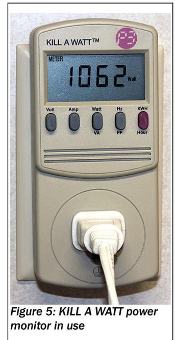
Figure 5: KILL A WATT power monitor in use
