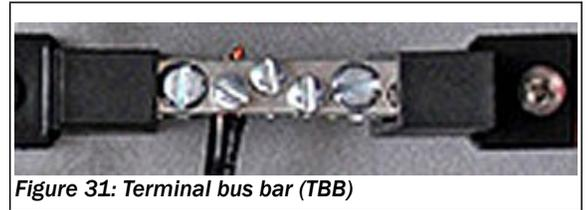
Figure 31: Terminal bus bar (TBB)
